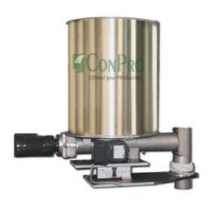
For weighing and dosing of materials it is necessary to keep the material output constant. The S/M-KTW-F has been developed in order to assure constant output for poorly flowing materials. An integrated agitator avoids bridge forming and provides a permanently filled dosing screw. The unit weight is calculated via a platform load cell. Via weight reduction values the throughput is calculated and controlled.
