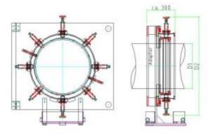
The measuring chamber type MH is flange mounted at the back side of the vacuum resp. cooling tank.
