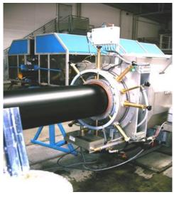
The monitoring and measuring of plastic pipes is carried out by ultrasonic. The measuring chamber type MH has a foldaway design and is flange mounted to the back side of the vacuum tank or cooling tank. Due to the hinge device the sealing
