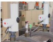
The monitoring and measuring of plastic hoses and tubes is done with ultrasonic. The sensors are fixed in the working position.
