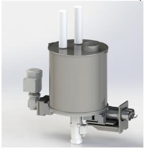
For weighing and dosing of materials it is necessary to keep the material output constant. The S/M-KTW-SD has been developed in order to assure constant output for poorly flowing materials. An integrated agitator avoi bridge forming and provides a permanently filled dosing double spiral. The unit weight is calculated via a platform load cell. Via weight reduction values the throughput is calculated and controlled.
