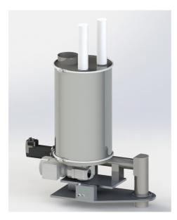
For weighing and dosing of materials it is necessary to keep the material output constant. The S/M-KTW-FS has been developed in order to assure constant output for poorly flowing materials. An integrated agitator avoids bridge forming and provides a permanently filled dosing screw. The unit weight is calculated via a platform load cell. Via weight reduction values the throughput is calculated and controlled.
