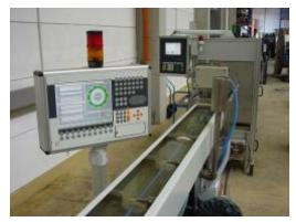
**SoniCon SL / MRR** is a multi applicable ultrasonic measuring and inspection system to control and regulate the production of hoses, cable and pipes (up to Ø 110 mm). The system is flange mounted downstream from the vacuum resp.cooling tank or it is integrated in a water tank.
