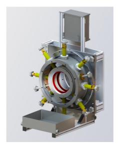
The monitoring and measuring of plastic pipes is carried out by ultrasonic. The measuring chamber type MH has a foldaway design and is flange mounted to the back side of the vacuum tank or cooling tank. Due to the hinge device the sealing exchange can be effected easily.
